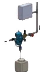
tank feed installation
